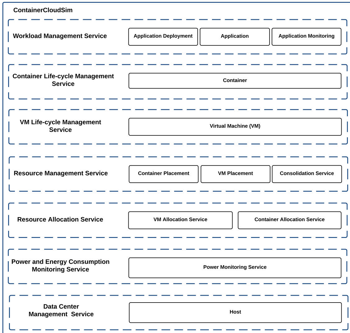
Figure 4.3: ContainerCloudSim simulator architecture.
