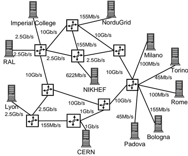
Fig. 10. The simulated topology of EU DataGrid TestBed 1
