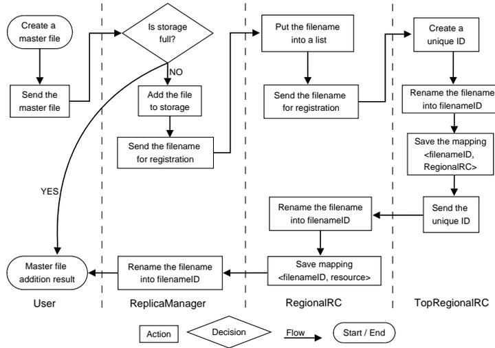
Fig. 6. Flowchart diagram for adding a master file
