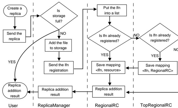
Fig. 7. Flowchart diagram for adding a replica
