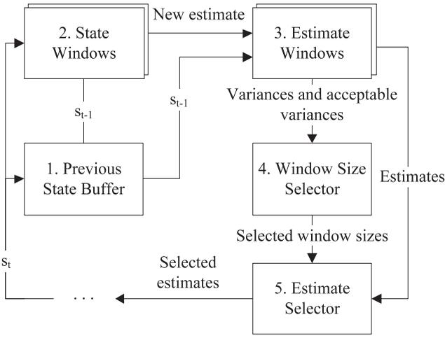
Fig. 1. The Multisize Sliding Window workload estimation.
