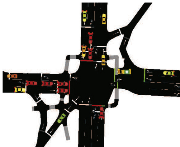
Fig. 10. Scenario 1: Traffic Network for six RoadSegments with two lanes in Sumo Simulation.
