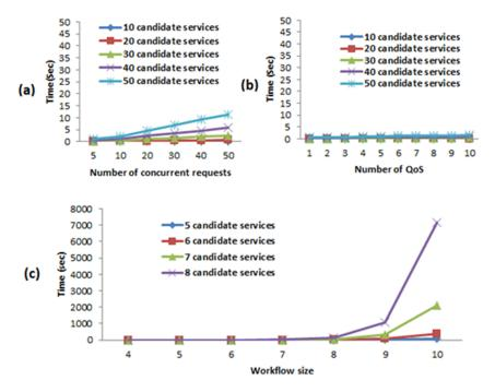
Fig. 16. The execution time of the portfolio-based composition as both of the number of candidate services and (a) number of requests, (b) number of QoS, and (c) workflow size increases.
