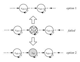
Fig. 16. State recovery for a failed stateful vertex.
