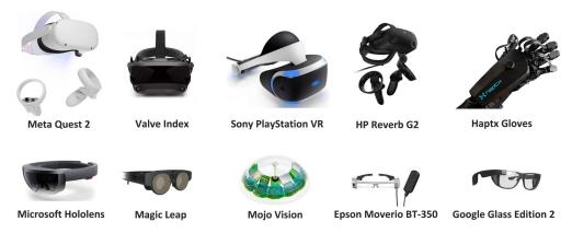
Figure 3: Metaverse wearable devices.
