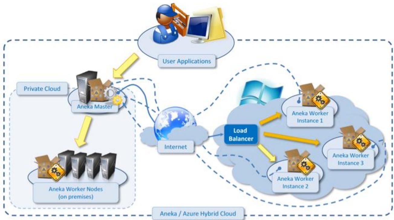
Figure 7: Schematic of Aneka/Azure Interaction for data analytics application
