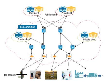
**Figure 1.** Distributed data processing in a fog-computing environment. Based on the desired functionality of a system, users can deploy Internet of Things sensors in different environments including roads, medical centers, and farms. Once the system collects information from the sensors, fog devices—including nearby gateways and private clouds—dynamically conduct data analytics.
