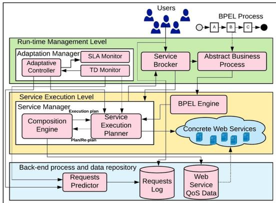
Fig. 2. The architecture of DebtCom.
