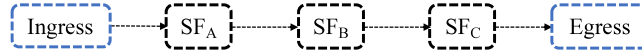
Fig. 8. The prototype SFC to evaluate simulation accuracy. Note that SF_A , SF_B and SF_C are chosen from the SFs listed in Table 2. In experiment 1 and 2 of Section 5.1, SF_A , SF_B and SF_C are Firewall, Logger and DPI respectively. While in experiment 3, we use Compressor and Decompressor as SF_B and SF_C .
